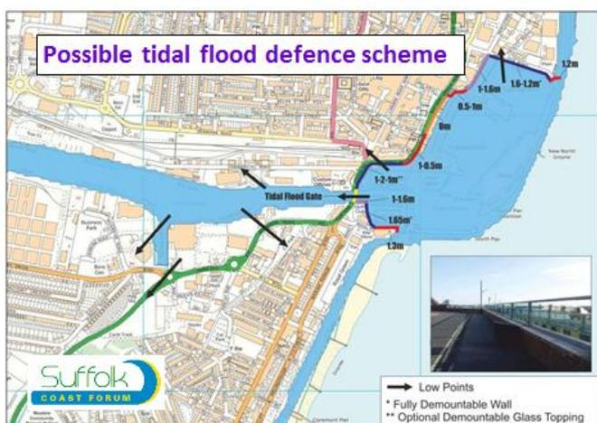
*Schematic showing extent of flood risk and possible tidal defence scheme for Lowestoft – details currently being progressed.*
